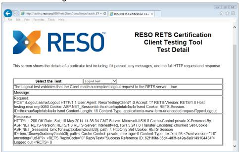
The Test Detail Page displays the details of the test, included the HTTP request and response.
